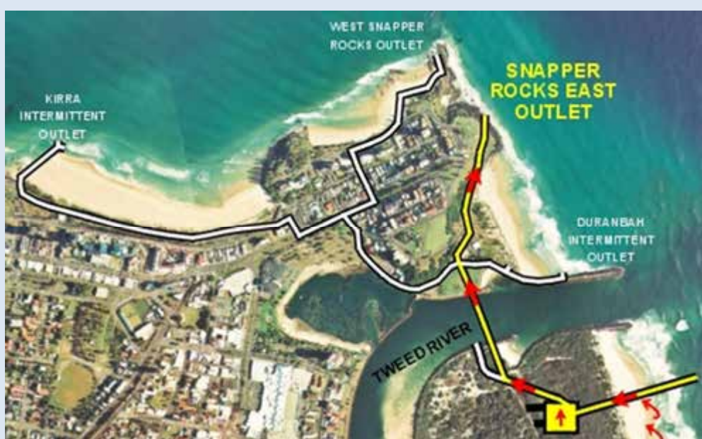
Figure 3 Sand bypass system of the Tweed River.
