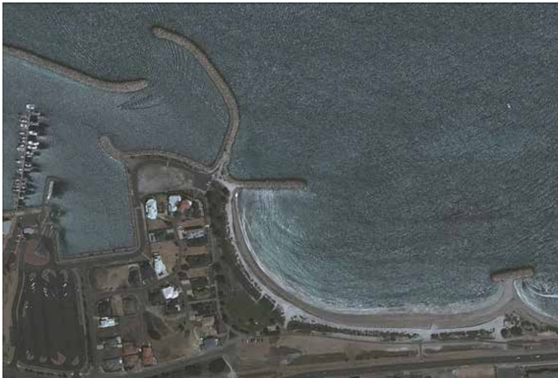
Figure 21 Detached breakwater (bottom right) forming a tombolo in Geraldton, Western Australia, as part of a coastal protection and harbour configuration Source: Google Earth
