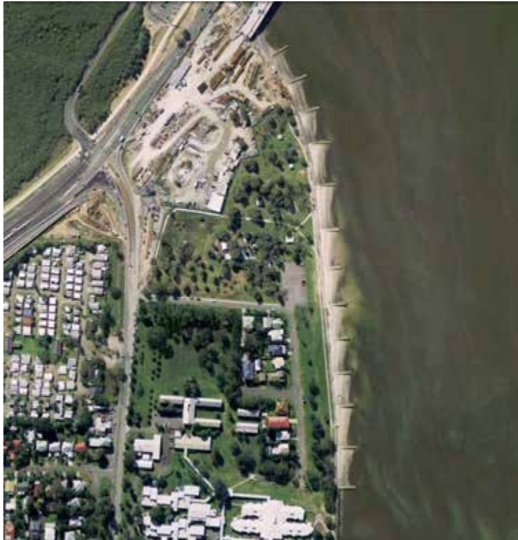
Figure 26 A groyne field and a seawall protecting settlements in Brighton, Moreton Bay Source: Google Earth
